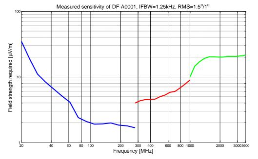
The graph illustrates the direction finding sensitivity of a typical system measured under specific electrical conditions.
